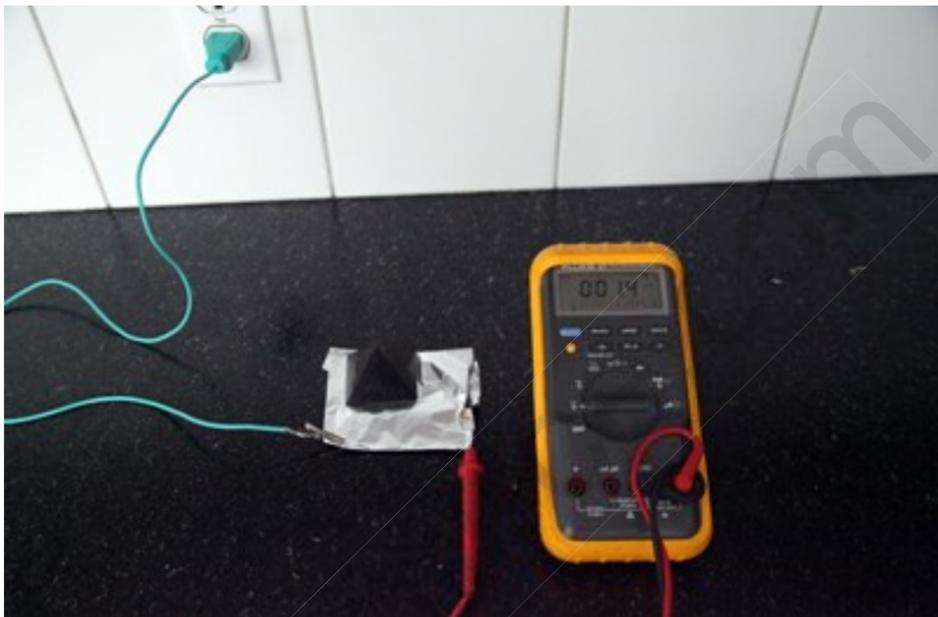
The Grounding Plug fits in any outlet in North America and has 3 prongs. Only the ground plug is active. The other 2 prongs are dead and not connected to anything. They will not provide any electric current from the outlet. They are used for a safety precaution.
