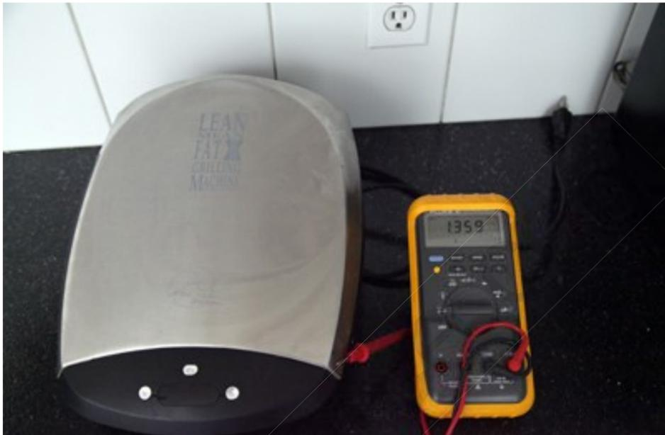
In the picture above the stainless steel appliance is not plugged in so it is not grounded and will not work to ground shieldite. We can see on our volt meter we have reading of 1359 milli volts. This is NOT grounded.
