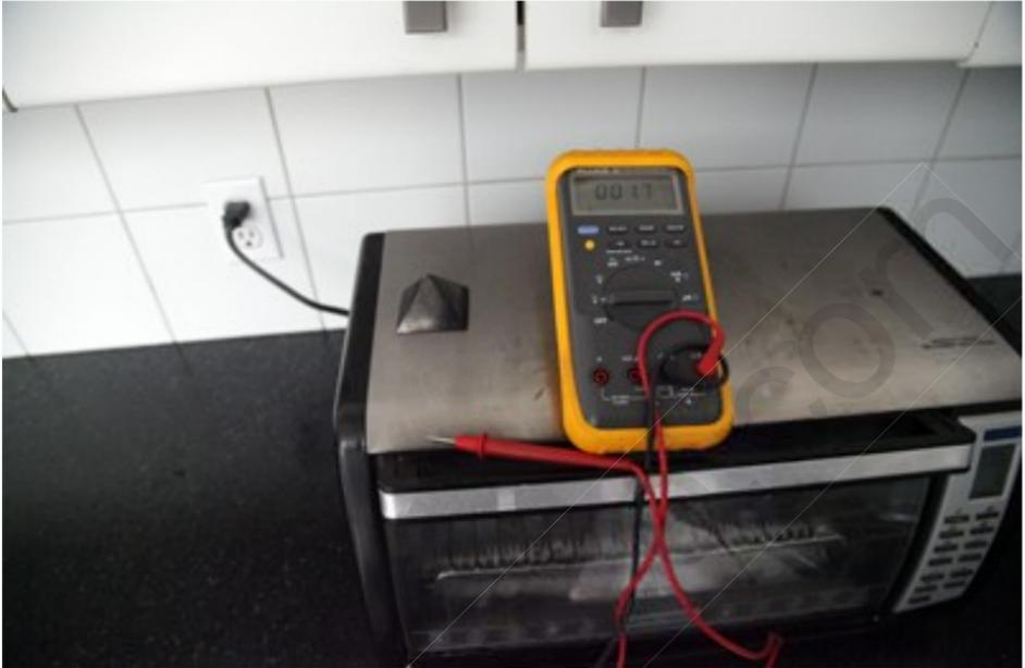
In the picture above the stainless steel appliance is plugged in, has a 3 pronged plug and our shieldite is touching the stainless steel on the appliance. We are testing it with our volt meter and have a reading of  $< 2$  milli volts which shows our shieldite is being grounded.
